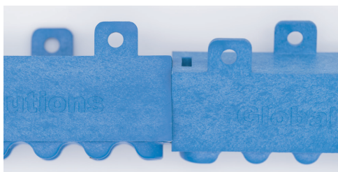
FIGURE 12B - Screw misaligned
