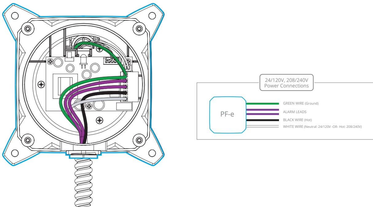
For your convenience and flexibility of installation the Pf-e is supplied without an electrical conduit and wire. It has a hole sized for ½" trade size conduit fittings (1/2" NPT) and an internal strain relief clamp.
