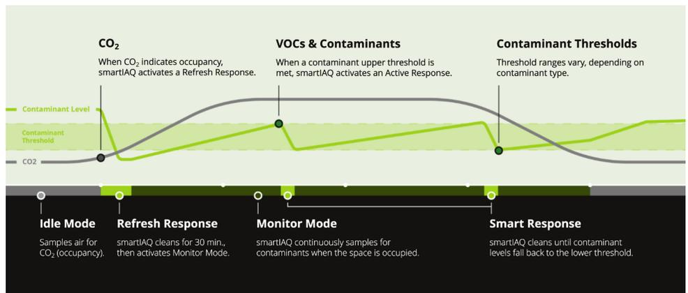
CO<sub>2</sub> is used to determine space occupancy, thereby aligning cleaning to times when people are present.
